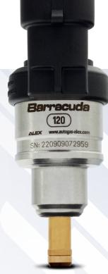
Barracuda 120 NI/min injectors are available in a version for single assembly - with or without an adapter (a connector for self-assembly), and combined into 3 and 4-cylinder rails. Removable calibration nozzle enables smooth adjustment of gas flow and injector efficiency (from 20 to 50 HP per cylinder). A single slim injector can be mounted close to a gasoline injector on a hose with a minimum length, which increases the **precision of gas injection**.
