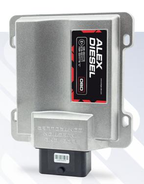
The ALEX DIESEL system is based on the mixing of 2 fuels: diesel oil and gas. The controller limits the injection of diesel oil to the amount that allows self-ignition in the cylinder, and in its place gives a precise dose of gas. The share of gas in the ALEX DIESEL installation is on average up to 30% LPG or 50% CNG. Such proportions of additional fuel guarantee the correct operating conditions of the engine and the entire system.
